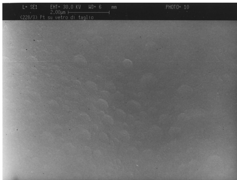
Figure 2 SEM micrograph of the morphology of platinum deposited on glass.
